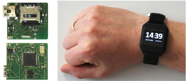
**Figure 2.** Our custom-made sensor platform, designed to be worn and used as a wrist watch, is light-weight enough to be worn for recordings of up to 2 weeks. Left: board with controller, accelerometer, micro-SD storage, and USB connector for data access and charging the battery.
