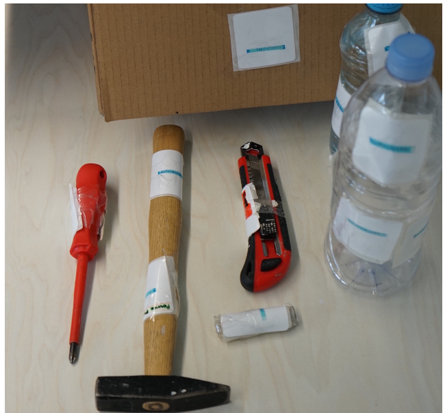
Figure 5: Selected items used in the experiment were tagged with RFID tags and were chosen to be similar with the objects reported in [3].
