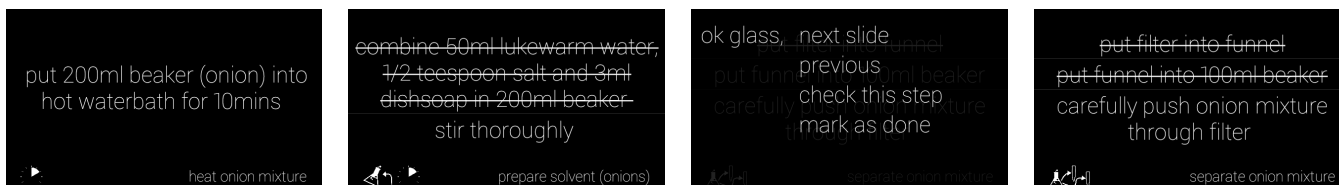
Figure 2. Examples of the user interface as presented to the participants while performing the study. Information cards are switched backwards and forwards, the current step can be marked as complete using speech commands. The second and fourth images are examples of checked /marked steps.
