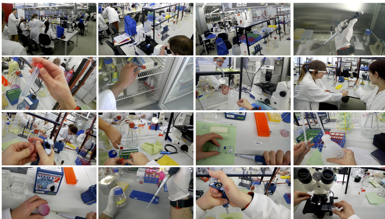
Figure 4. The deployment of the system combining Glass and the wrist-worn accelerometer, while continuously recording researchers at work in a wet lab. The environment is often simultaneously used by large groups of researchers or students and is equipped with a multitude of shared instruments and special safety zones, making it challenging to augment the environment (top half). Hands-free recording is a strong advantage: Often, experiments require gloves for minimizing contamination risks; Wet labs furthermore contain a large variety of compounds, instruments and lab equipment that require both hands to be used (bottom half). All these photos are unaltered frames taken from continuous Glass video recordings.
