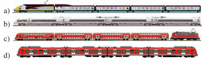
Fig. 5: The four passenger train types in the data set, from above: a) Thalys, b) ICE, c) Regio, d) CityRail. Note that the trucks’ locations differ among the train types, with two trucks for a wagon (e.g. ICE) or one between them (e.g. CityRail), resulting in characteristic vibration footprints.
