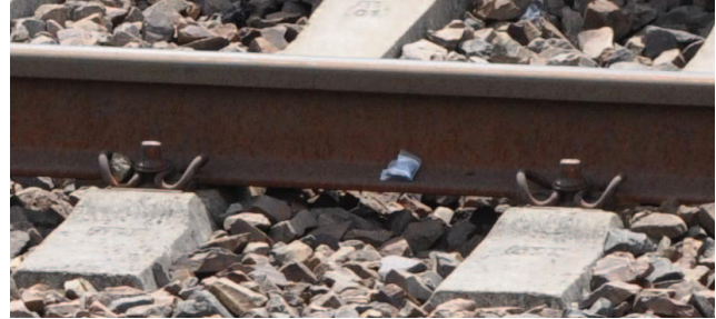
Fig. 3: One of the sensor nodes attached to the rails during the experimental deployment. The sensor node is wrapped up in a plastic bag to protect the sensor from dust and humidity.
