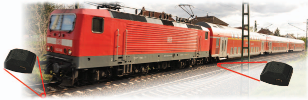
Fig. 2: Our system’s concept: A sensor network deployed along railway tracks captures vibrations caused by passing trains. Immediately computing efficient features from streaming sensor data allows train type classification and counting wagons on the sensor nodes. In future deployments, these can be used to estimate train speed and detect worn-down cargo wheels. As such, this system is envisioned as a flexible instrument to assist in railway monitoring and maintenance tasks.
