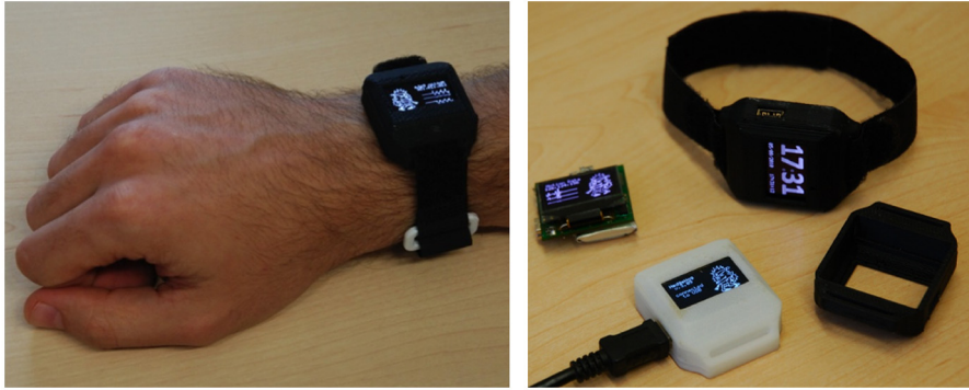
Fig. 4. HedgeHog is a device worn like an actigraph at the dominant wrist records motion, posture, and light data over a long time-span.
