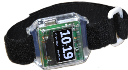
Fig. 1: The custom-made inertial data logger was designed for long-term (day and night) recording of data for activity recognition at 100 Hz, while simultaneously taking user acceptance requirements for wearing such as device into consideration. We focus on the evaluation of low-power design choices.
