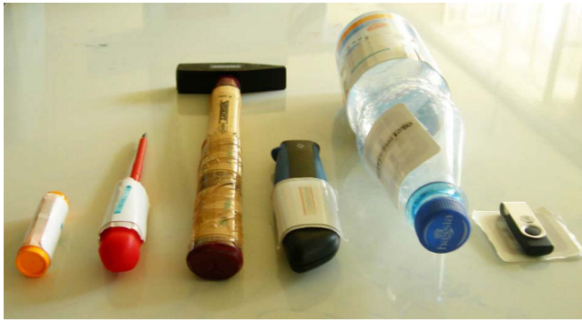
Figure 4. Some of the objects from the box test, chosen to have a high variety in shape, weight and material, tagged with RFID tags.
