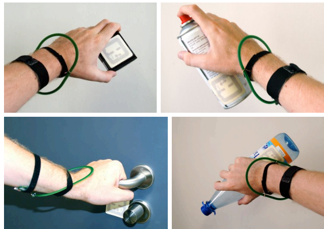
Figure 1. The wrist-worn prototype identifies grabbed objects and the physical interactions with them, using a combination of RFID and inertial sensors. This paper's aim is to explore light-weight and power-efficient solutions in particular, to facilitate long-term deployment.
