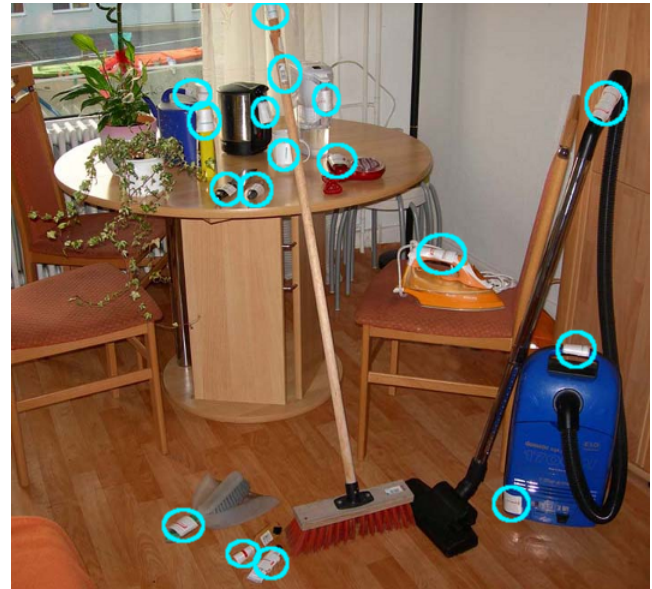
Figure 12. Some of the objects from the longer-term domestic setting study. Tagged objects and tools were chosen for their interactions, whereby 43 tags have been deployed, and scattered around the living environment of the test subject.
