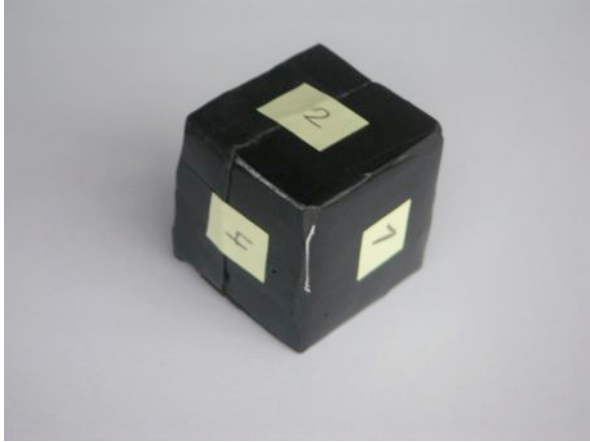
Figure 9. Labels were attached to the cube in the experiment to allow cross-checking between the real outcome (“face 2” in this case) and the one classified by the die.
