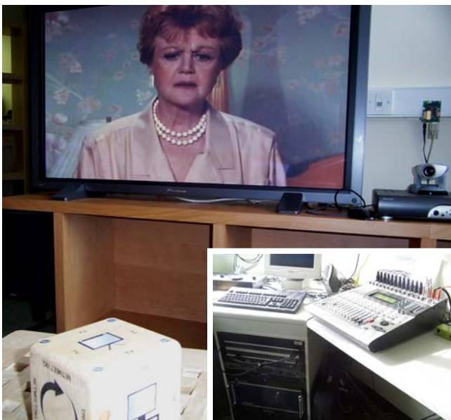
Figure 10. The cube that selects audio profiles for the lab’s mixer panel has labeled sides corresponding to the available audio sources. The side on top (TV in this case) is selected. The small circuit board above the camera to the right of the plasma screen is the base station. The inset shows the equipment that drives the lab’s audio system; sliders and channels are automatically set to one of six common profiles by the cube.
