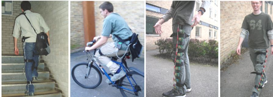
**Fig. 6.** Experiments of [10] with networks containing a large amount of motion sensors: the left two using 40 accelerometers, the right two using 90 tilt switches.
