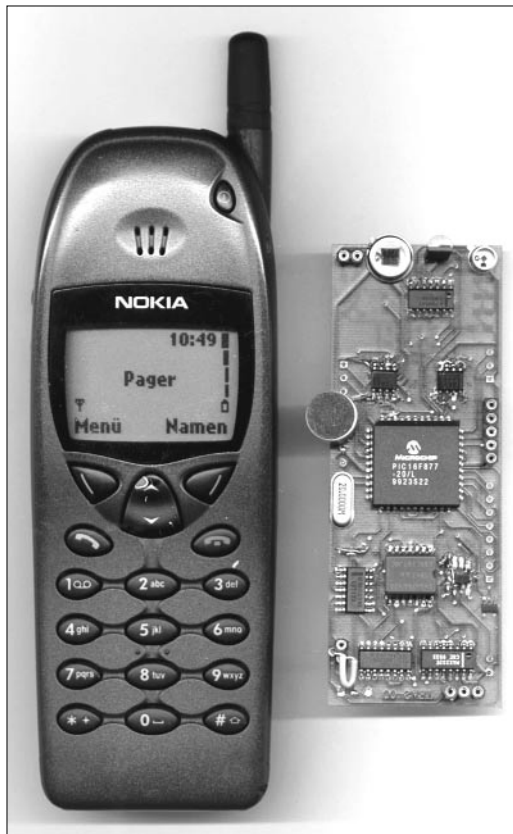
■ Figure 2. The sensor board and the enhanced mobile phone prototype.
