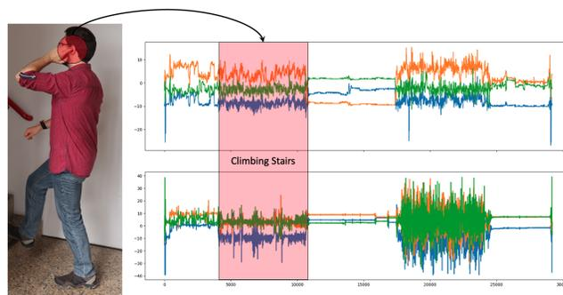
**Figure 1:** We present an inconspicuous annotation method, in which users can annotate their activity data *in situ* with an in-ear wearable (left), to mark and synchronize inertial data from the ear with all other inertial sensors (right).
