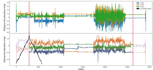
**Figure 3: Best synchronization with a mismatch of 0.30 seconds. The figure shows that the synchronization works best with sufficient long periods of sedentary activity. The inertial signal of the wrist (top) compared with the synchronized signals of the head (bottom). The black signal at the bottom left depicts the cross-correlation between the binary filtered signals.**
