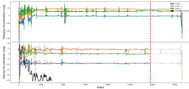
**Figure 5: Worst-case synchronization with a mismatch of 34.84 seconds, record 14 in table 3. In this data almost only desk work has been performed. The inertial signal of the wrist (top) compared with the synchronized signals of the head (bottom). The black signal at the bottom left depicts the cross-correlation between the binary filtered signals.**
