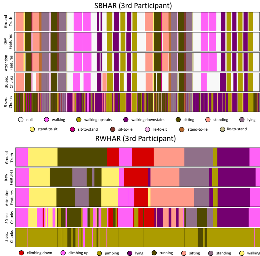
Fig. 7. Color-coded visualization of the effect of the Offline and Online Activity Recognition experiments using the ActionFormer model [66]. Results are compared with the ground truth of a sample participant as well as offline single-stage training for both the RWHAR [50] and SBHAR [43] dataset. One can see that training the TAL models using attention based features clearly improves results with an overall better recognition of all activities. Contrarily, once predicting a chunked output, performance can be somewhat maintained for larger chunks, yet drops near zero once applied on only 5-second long windows.
