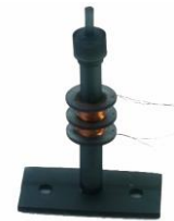
Figure 4. Improved setup with two coils, with n=700 , wire diameter d=0.1\text{mm} , h_c = 4\text{mm} , 4 mm magnet.
