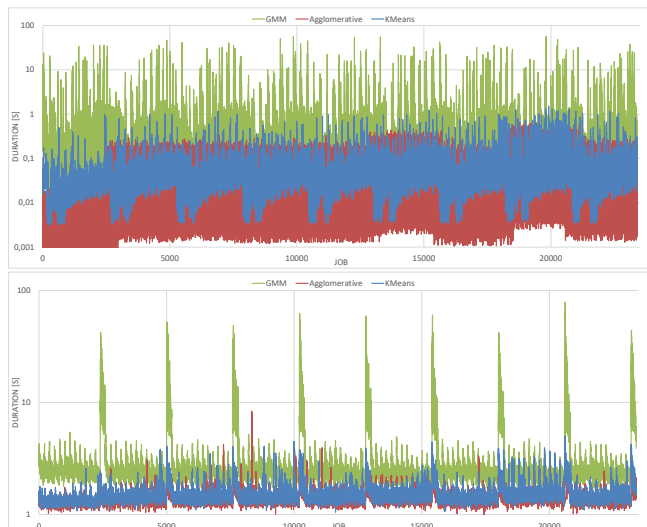
Figure 5. Process benchmark of the CMU kitchen experiments (y-axis log-scale). Durations (in sec) of only the clustering process (top), as well as the whole experiment run (bottom), including preprocessing and feature extraction, are shown. Benchmarked algorithms are KMeans (blue), agglomerative clustering (red) and GMM (green).
