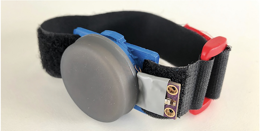
Fig. 2. Our prototype consists of a Puck.js with the attached BME280 sensor. A custom 3D-printed enclosure can be mounted on the wrist using the wristband.
