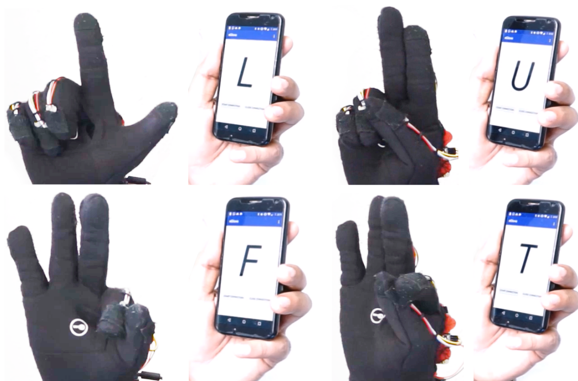
Figure 1. This article's self-contained data glove is capable of detecting and distinguishing between fine-grained signs in real-time through a set of miniature IMU units, one per finger. Detection is performed on an integrated system placed in the back of the glove, powered from a flat Li-Po battery integrated under the wrist. Shown are four different gestures (out of the 22 we consider in the evaluation) including those that for most gloves are not easily distinguishable from each other.
