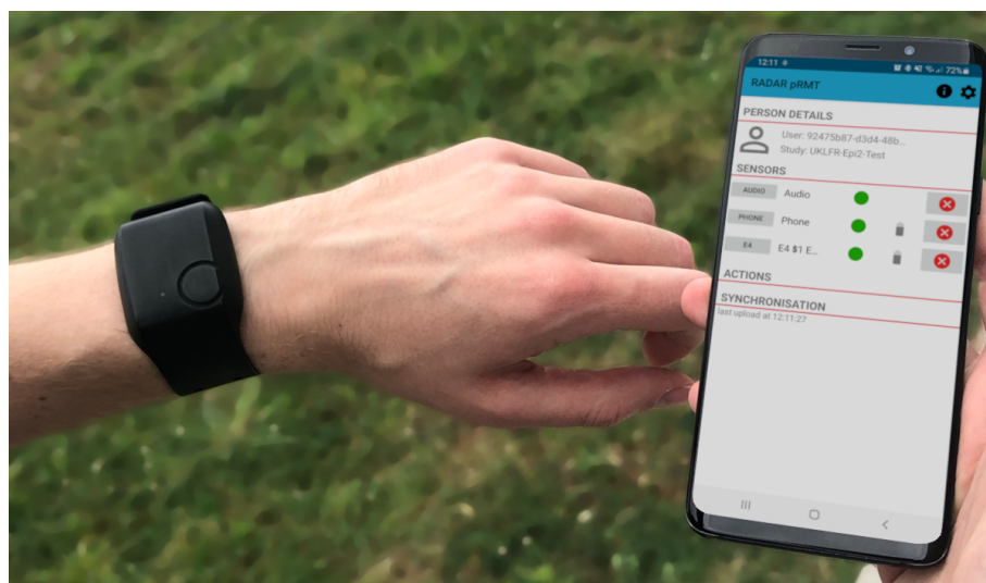
Figure A1. The Empatica E4 wrist-worn wearable device used in this study (left), and the Android phone application that connects to the wearable via Bluetooth and records the data stream (right).
