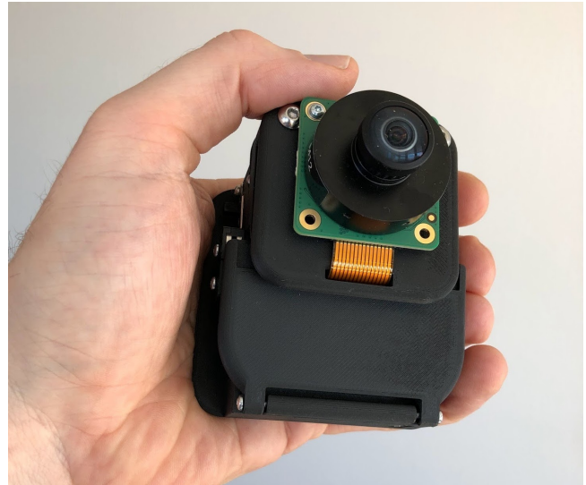
Figure 1: A fully assembled ChronoVault prototype, which has the form factor of a clip-on module with wide-angle front-facing camera and large-surface button (bottom front).
